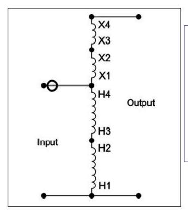
Input Voltage = 208 V Output Voltage = 236 V
